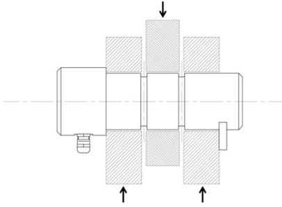
*Load Pin using the Double Shear Measurement Principle*
