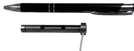
*An externally strain gauged load pin.*
