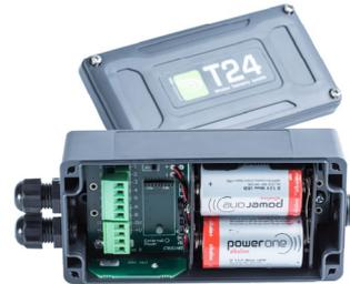
The T24-ACM is the largest of the transmitter enclosures. Featuring a compartment for a pair of alkaline 'D' cells, the T24-ACM also has a regulator circuitry for an external power supply. The batteries can also be used to provide power in case of external supply failure.
