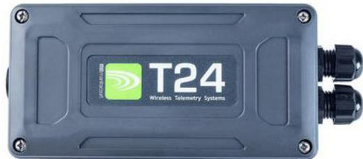
The T24-RM1, wireless receiver with relay output, offers dual power relays capable of mains power switching. Each relay can be configured as high, low or window alarms and can be associated with a group of up to eight T24 transmitters.
