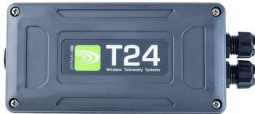
The T24-GW1 is a wireless Modbus\* gateway that provides a simple interface for users to gather data from up to 100 transmitters in a T24 network. The T24-GW1 uses either the standard Modbus interface RTU protocol or a simple ASCII protocol.
