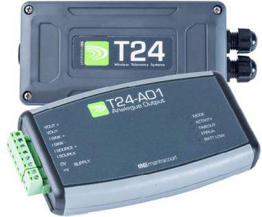
The T24-AO1 provides a configurable analogue output for a single T24 wireless transmitter module. The output can be selected from the pre-calibrated voltage and current ranges of 0-10 Volts,  $\pm 10$  Volts, 0-5 Volts,  $\pm 5$  Volts, 0-20mA and 4-20mA. (All current outputs both sink and source).
