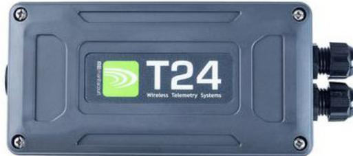
The T24-BSi is housed in an IP67 enclosure. Data can also be captured by the wireless telemetry base station (T24-BSi) from an unlimited number of T24 transmitter modules. Whilst the integral antenna on the T24-BSi offers up to 800m range in an open field site.
