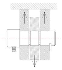
Typical Load Pin Installation
