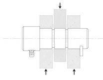
Load Pin using the Double Shear Measurement Principle
