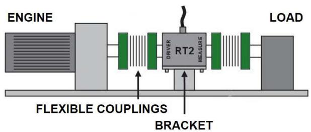
The RT2 measures CLOCKWISE torque with a POSITIVE output in tension or ANTICLOCKWISE torque with NEGATIVE output in tension.
