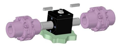
The assembly of the couplings to the RT2 must be done whilst disconnected from the machine (system) with the transducer only connected to a display, thus verifying in real time that no unwanted torque, bending or tension are generated which may overload the transducer.
