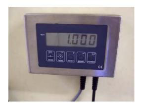
Display: 6 digits, 18mm high LCD or LED displays
