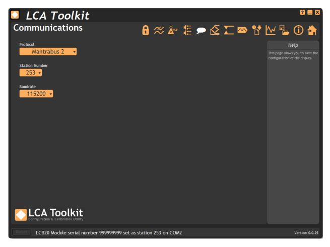
**Protocol** - Select the required communications protocol. All modules on the same communications bus should be set to the same protocol.
