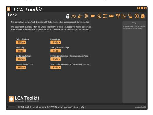
Certain pages and functionality can be hidden or disabled using this page. Once the LK2 jumper link is removed and the module is connected to the LCA Toolkit this page and all other selected pages and functions will be hidden.
