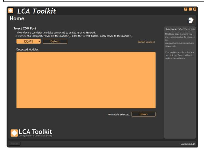
The serial ports (COM ports) on the computer are detected and added to the drop down list on the top left of the page. If you are using USB to RS232 or RS485 convertors then you can plug them in at this point. Clicking the drop down list will automatically re-detect available COM ports.
