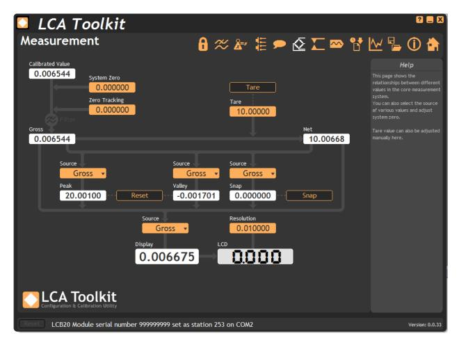
**Calibrated Value** - Shows the calibrated value. Calibration turns the input mV/V value into this value.
