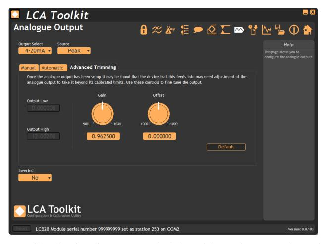
**Gain** - Alter the analogue output gain by clicking and dragging the pointer on the virtual knob.
