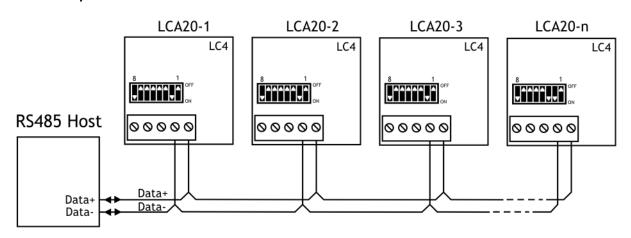
The last LC4 module in the 'chain' has DIP switch position 3 set to On
