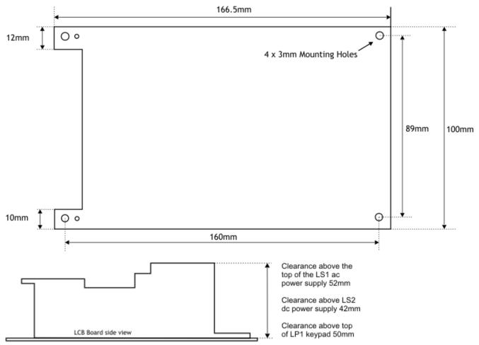
Clearance below the board should be 3mm. If it needs to be insulated allow 6mm.
