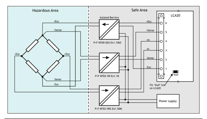
Because the barriers are fully isolated, the **Vref** link <u>MUST</u> be fitted to ensure that the LCA20 input stage is biased correctly.
