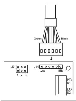
Please ensure correct orientation as marked by colour coding on LCA20 PCB
