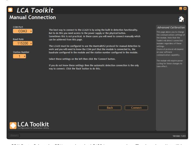
**COM Port** - Select the COM port that the LCA20 is connected to. The drop down list will be populated with all detected Com ports.
