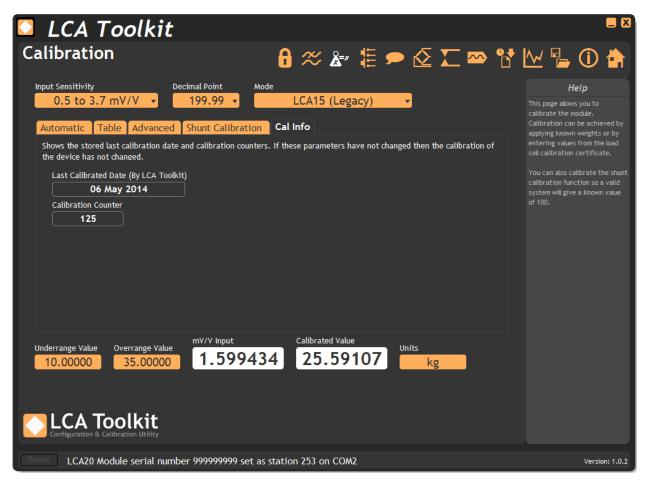
**Last Calibrated Date** - Indicates the last date that calibration was performed by the Toolkit. **Calibration Counter** - Shows the internal calibration counter.
