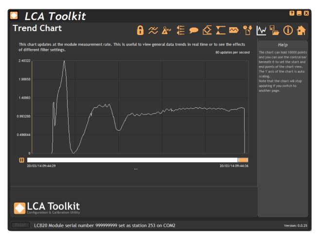
**Pause Button** - Pauses the chart. During a pause no more data will be added to the chart. You can use the range scrollbar to change the view or click and drag on the chart to move the cursor. The time and value of the data under the cursor will be displayed under the chart.
