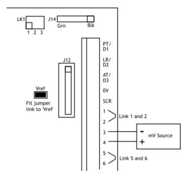
Fit the jumper link to the pins marked 'Vref'. See diagram above.
