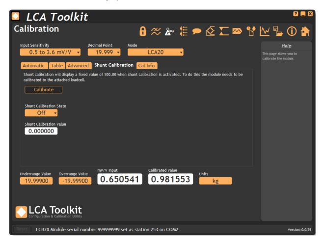
**Calibrate** - Click this button to calibrate the shunt to the current load cell attached.
