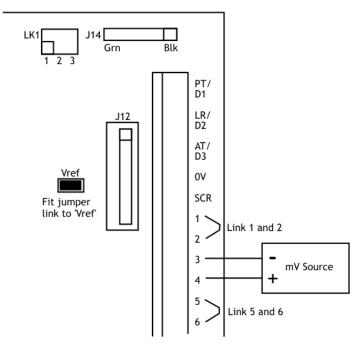
Fit the jumper link to the pins marked 'Vref'. Measure the Excitation voltage across 1 and 6 on the connector. Multiply by the mV/V values on the calibration certificate at the required calibration
