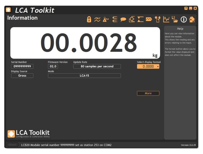
**Main Display** - Displays the module value. If units have been specified at calibration then the units will be shown.
