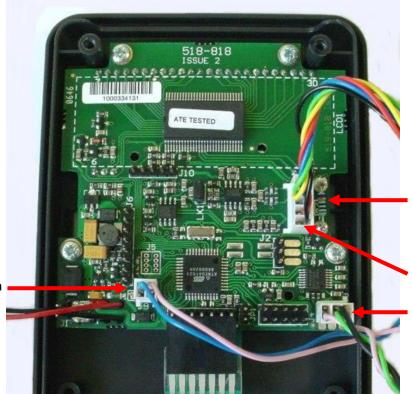
Shunt Calibration Resistor
